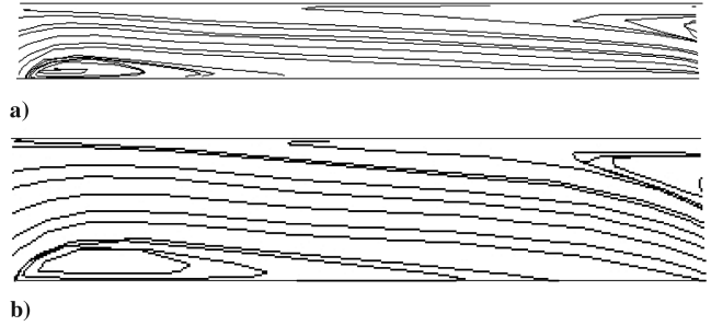
Fig. 6 Streamlines inside tip clearance region at t^* = 0.25 for a) case 1 and b) case 2.
